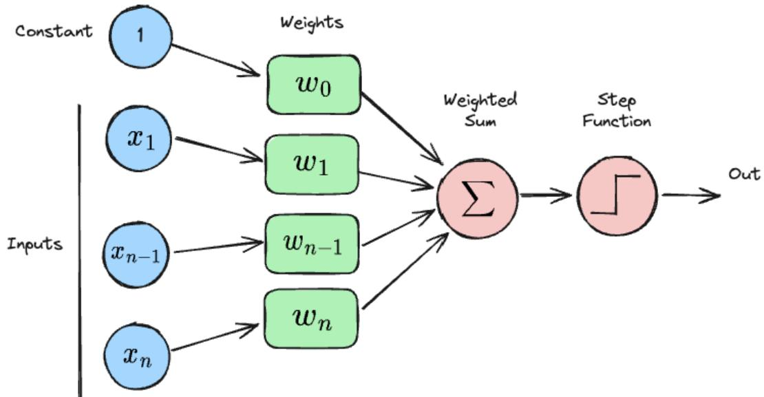
A logic gate is similar to a perceptron in that it also can be used as a binary linear classifier. With XOR, it takes on the implementation of a multi-layer perceptron, but the main concept within leveraging logic gates as perceptrons is that they both function as binary linear classifiers as demonstrated below:
